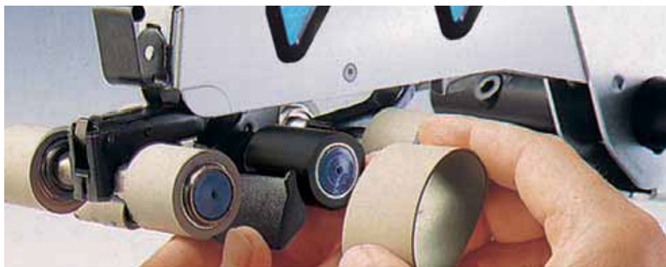
Easy apron exchange without removal of the top apron cradle: Top apron cradle with individual tensioning system.
